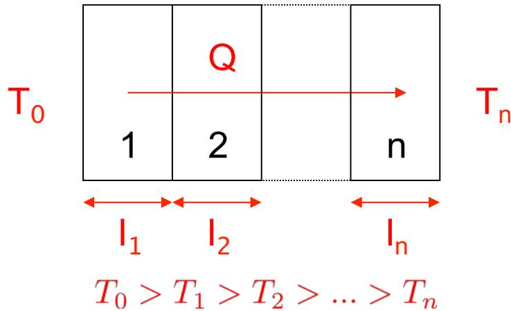
$$\frac{Q}{\Delta t} = A \frac{T_0 - T_n}{\sum_i \frac{l_i}{\kappa_i}} = A \frac{\sum_i l_i}{\sum_i \frac{l_i}{\kappa_i}} \frac{T_0 - T_n}{\sum_i l_i}$$
